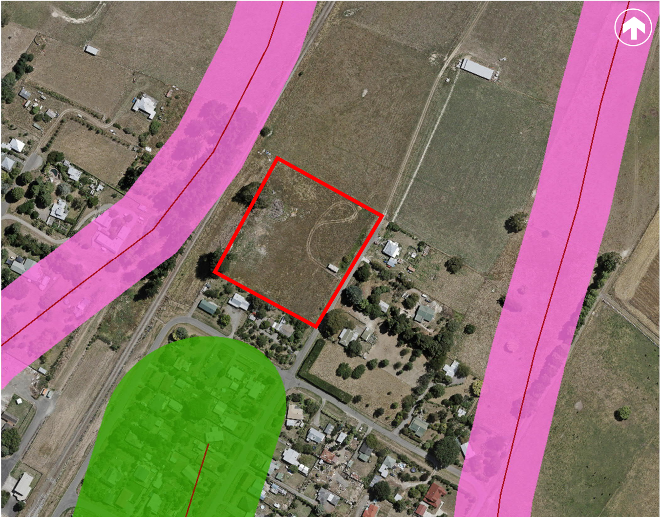
Figure 4: Aerial image showing the mapped faults in the immediate area of the site. The accurately mapped traces are shown in pink, with the distributed fault in green. (Source: Retrolens).
