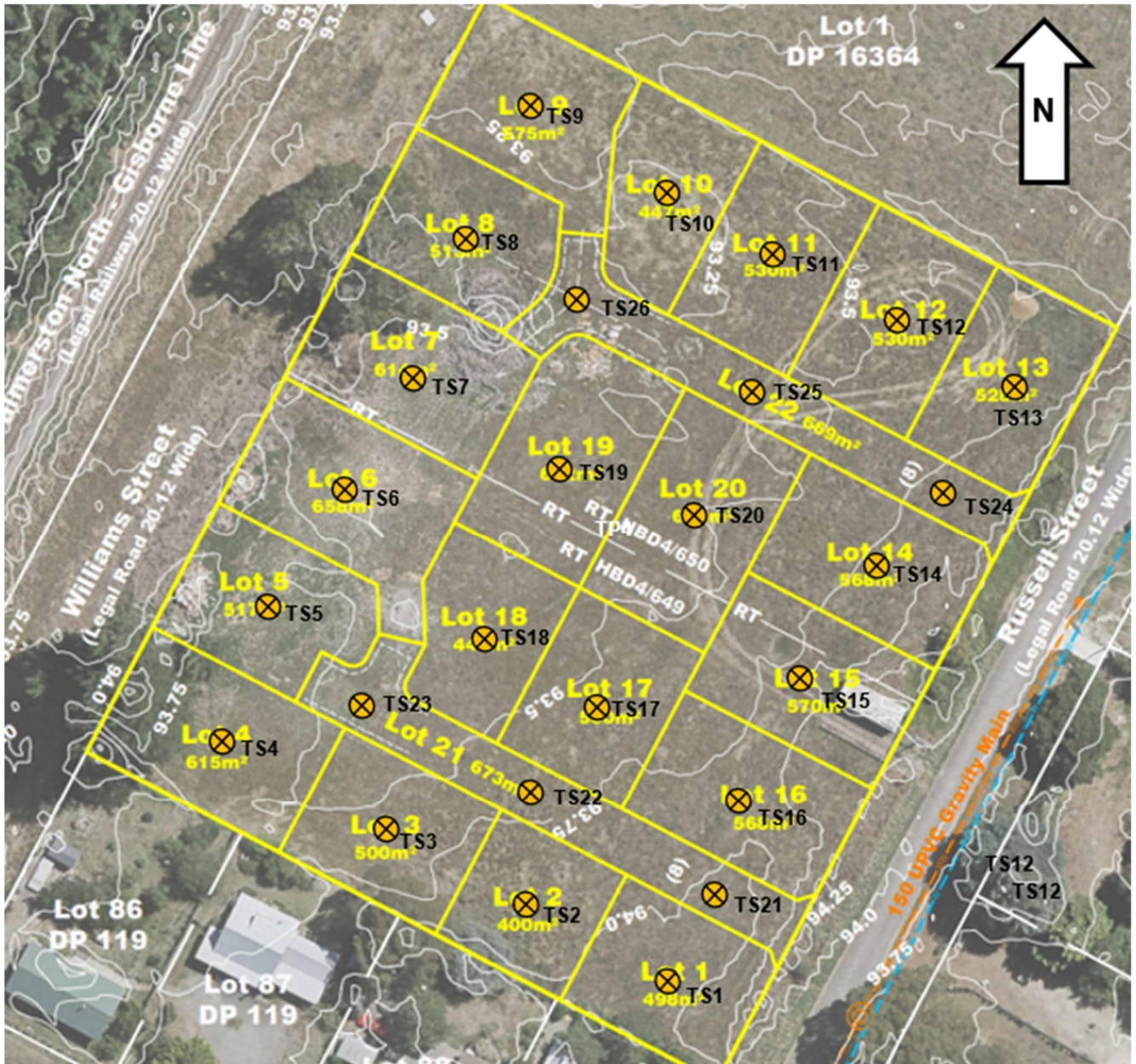
Figure 10: Scheme Plan showing the location of the Test Sites (TS) (Source: Surveying The Bay).
